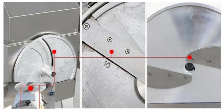
6. This blade is for dicing. First cut potatoes, and then cut it dices according to the size of dicing knife plate. Cutting size are 8mm, 10mm, 12mm etc.
