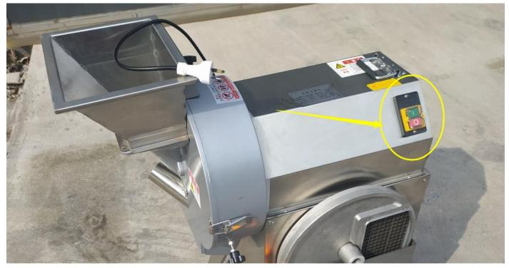
2. Large-caliber inlet for easy feeding. The cutting area for round-shape and roots vegetables and stems adopts a
